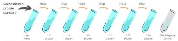
Two-fold dilution series: Each microvial starts with 10 Oul diluent. 100µl is carried over from the reconstituted protein standard, thoroughly mixed and then 100µl is transferred to the next. The process is repeated in each microvial in the sequence. No treatment is carried out on the negative control, which should hold 100µl of diluent.
