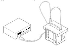
9. Disassemble the sandwich when the electrophoresis ends, take out the membrane and continue the next step. Use the neutral detergent to rinse the electrophoresis tank, blot clip, macroporous sponge, and then again use the ion-removing water to rinse.
