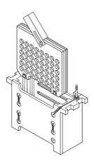
6. Put the cold cooling unit in the tank and fill up the tank by buffer.
