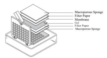
Note: In order to achieve the best blot result, it is key to remove the air bubble by glass bar stirring.
